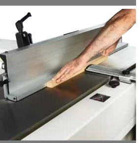
Additional overturning fence Integrated in the surface fence, it ensures perfect operator safety when machining small dimensioned work-pieces.
