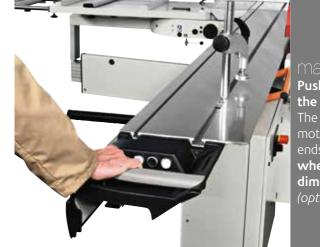
Pushbuttons integrated in the sliding carriage
